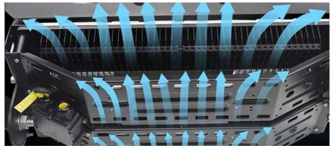
1060 Pure aluminum fins riveting design Hollow out in the middle of the heat sink increasing air convection, better heat dissipation.
