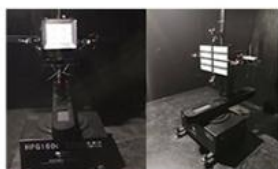
IES Photometric Testing
