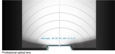
Different beam angles are optional: 30°/60°190\*120°1T2/T3/T4meeting the requirement of professional light distribution, restraining the dazzle light and spilling light effectively.
